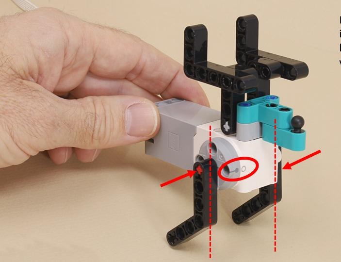
Make sure the motor is in its zero position and both front legs start vertically downward.
