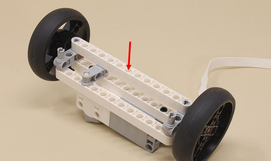
Make sure the wheels are aligned straight and the motor is in its zero position when you insert the axle. Push the axle all the way into the motor.
