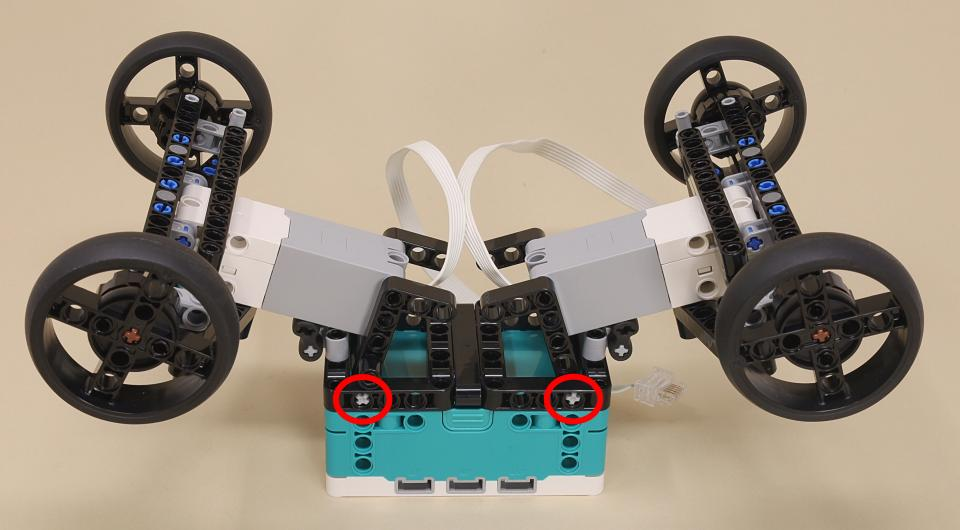
Twist the front steering motor clockwise until it stops with the wheels straight forward, then twist the rear motor counter-clockwise, to get the alignment shown.
