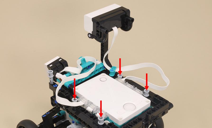
The arm wire should remain loose so the arm can unfold.
