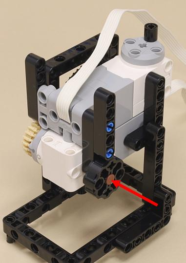
You can use this knob to adjust the turntable position manually.
