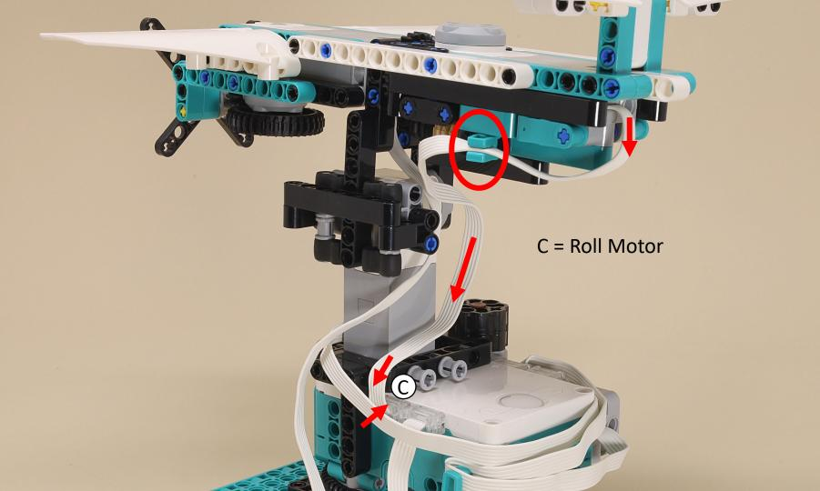
The airplane should be as level as possible, with the base aligned as shown when the motors are in their zero positions.
