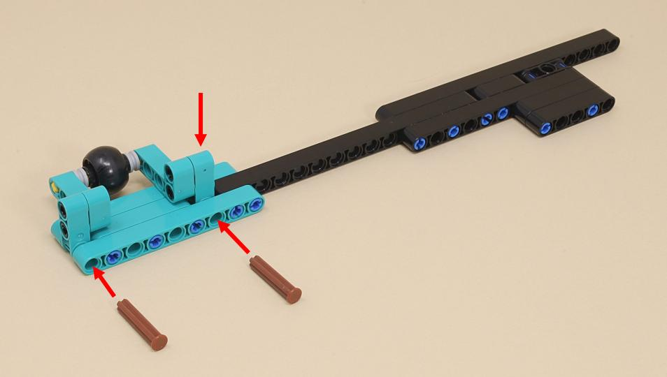
Check that the wheel spins freely. Loosen the bushings on either side of it if necessary.
