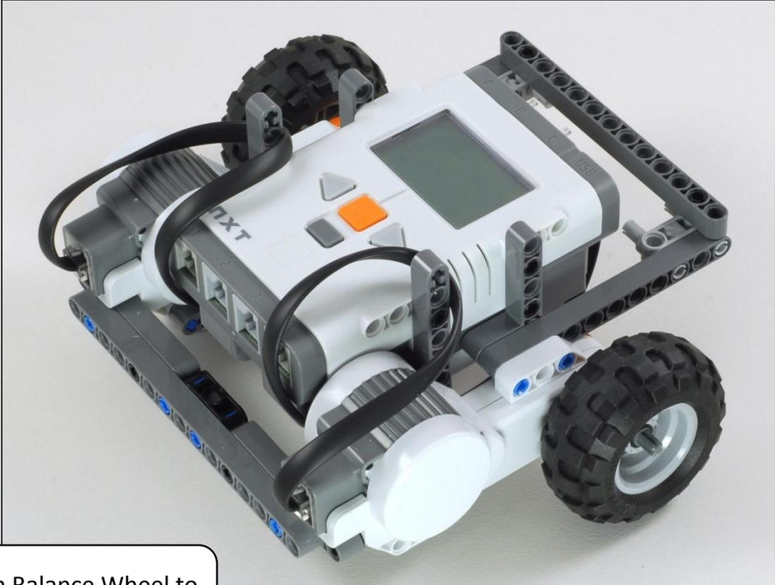
Add a Balance Wheel to make a complete robot.
